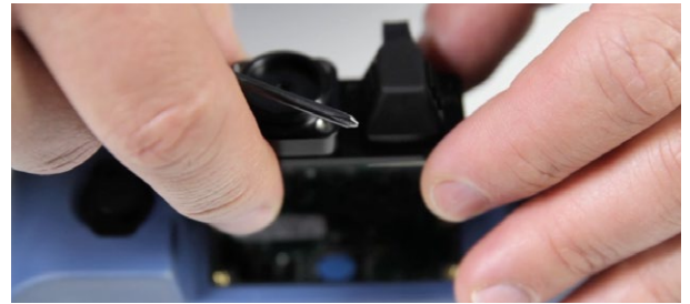
The easy-to-install power meter and VFL pieces attach to the MAX-FIP display using four screws.
