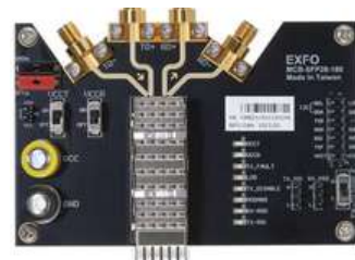
MCB-Module Compliance Board MCB to test next-gen transceivers
